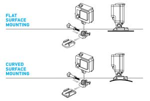
**TIP:** Apply adhesive mounts to clean, smooth surfaces at room temperature only, at least 24 hours before use. To remove, heat with a hair dryer then peel off mount.
